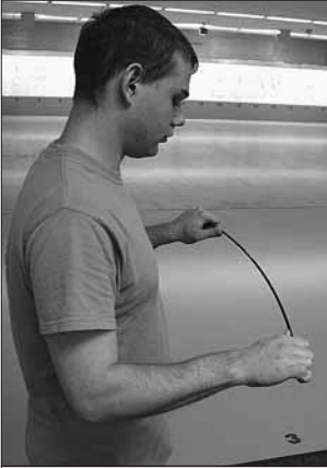
Checking a carbon arrow for cracks. There will be a grating sound if it is cracked.
